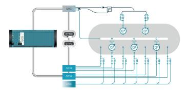
The QRC module is configured with other modules in the Cluster mainframe to obtain charge stability diagrams and drive qubit transitions while simultaneously supporting high-speed RF reflectometry measurements.
