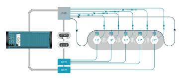
The QRC module is paired with the QCM module for flux pulse delivery, forming a fully integrated Cluster control stack solution for single and two qubit gates and resonator readout.
