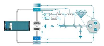
The QRC seamlessly integrates with the Qblox portfolio for color centers to combine qubit control, photon counting, and timetagging with feedback capabilities into a single mainframe.
